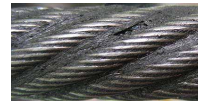
Left Lay - Counter Clockwise Rotation
